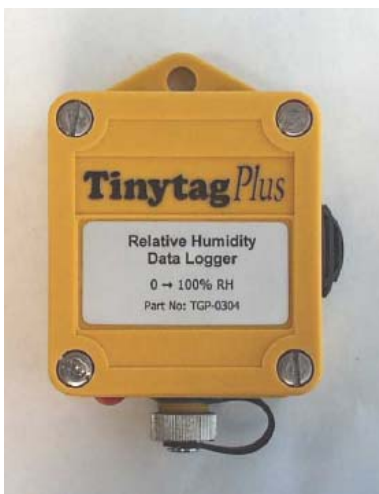
Figure 5: Tinytag Plus logger for measurement of external relative humidity
