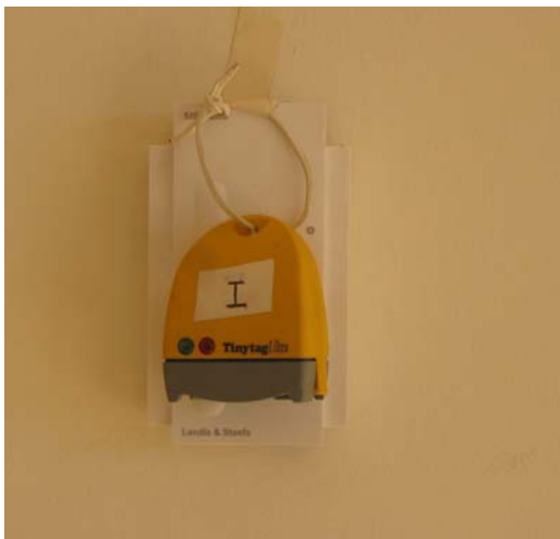
Figure 2: Tinytag logger for measurement of indoor air temperature and relative humidity
