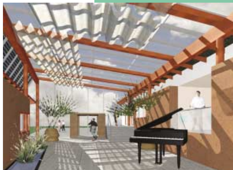
Shading system at Fachkrankenhaus Nordfriesland Hospital
